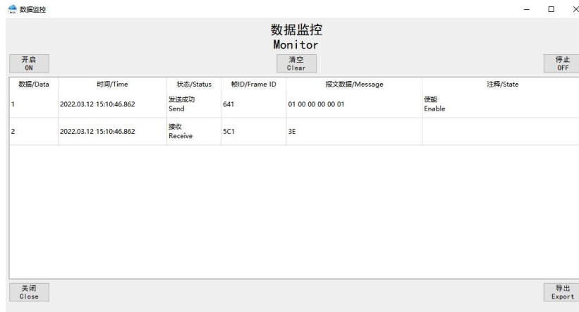
Figure 4-3 Monitoring Messages of “Enable”
