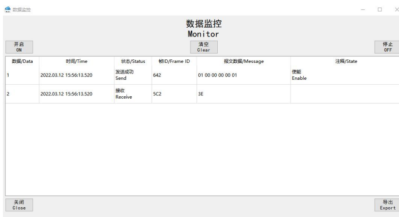
Figure 4-23 Monitoring messages of “Enable”
