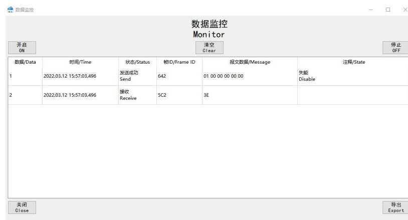
Figure 4-20 Monitoring messages of “Disable”
