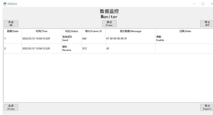
Figure 4-18 Monitoring messages of “Enable”
