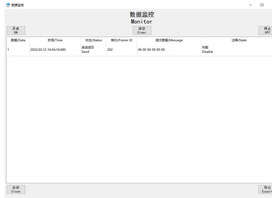
Figure 5-6 Monitoring messages of “Disable”
