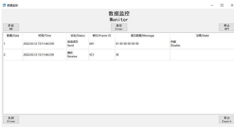
Figure 4-5 Monitoring Messages of “Disable”
